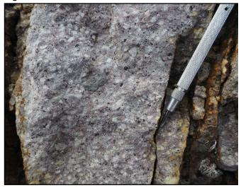
Example of unaltered andesite lapilli tuff. Variably broken plagioclase crystals and lapilli are common and reveal the pyroclastic character. Plagioclase crystals have obvious cleavage and are glassy. Lapilli are visible in the centre and top-centre of the sample. Unaltered andesite has distinctive purple-brown matrix.
