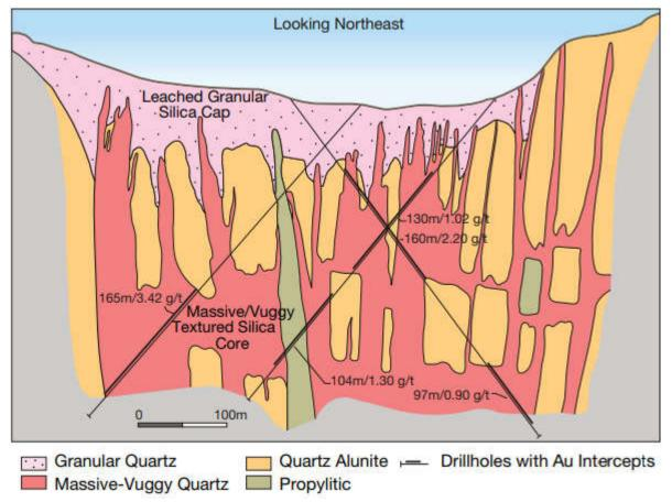
This section from Yanacocha illustrates the occurrence of gold in sub-vertical, massive/vuggy silica structures enveloped by advanced argillic alteration and capped by a leached zone of granular silica (Teal and Benavides, 2010).
